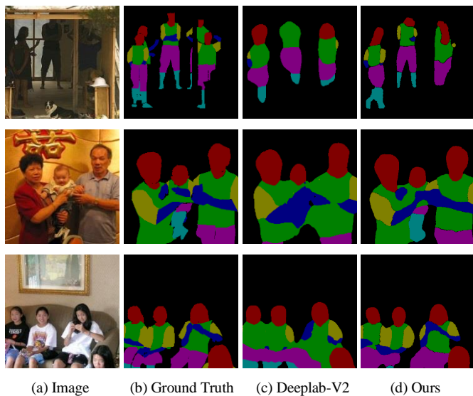
Figure 4: Segmentation results on the PASCAL Person Part Dataset proposed in [9], the input images are with multiple people.
