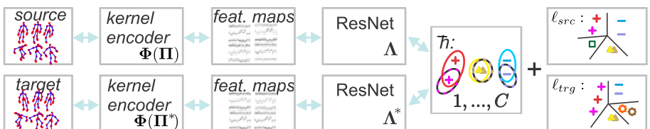
Figure 4: Our pipeline combines 3D body skeleton encoders with the supervised domain adaptation streams. Unlike [22], we utilize two classifiers (one per network stream) and perform alignment between the classes that are shared between the source and target datasets.
